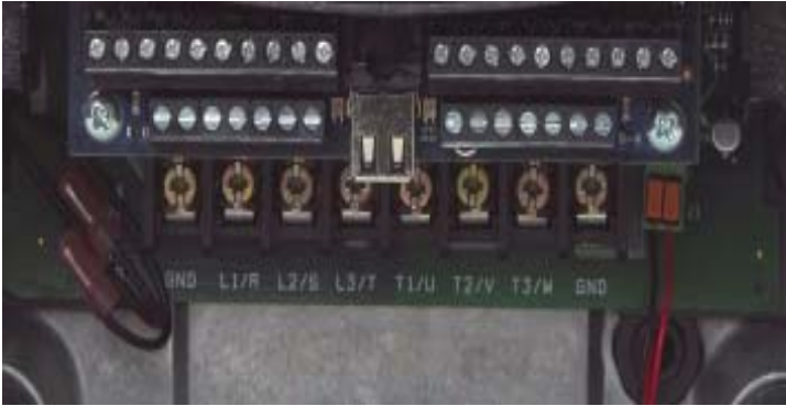
Figure 7: Vacon 500x Power Terminals
