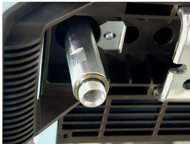
Figure 28. External thread of hose adapter
