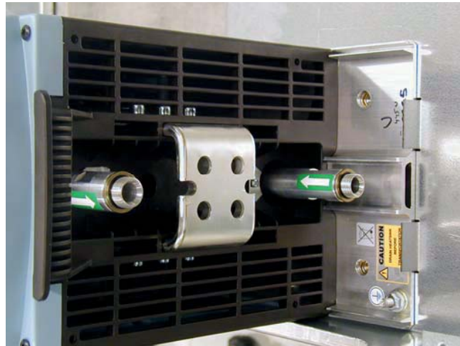
Figure 27. Aluminium hose adapters
