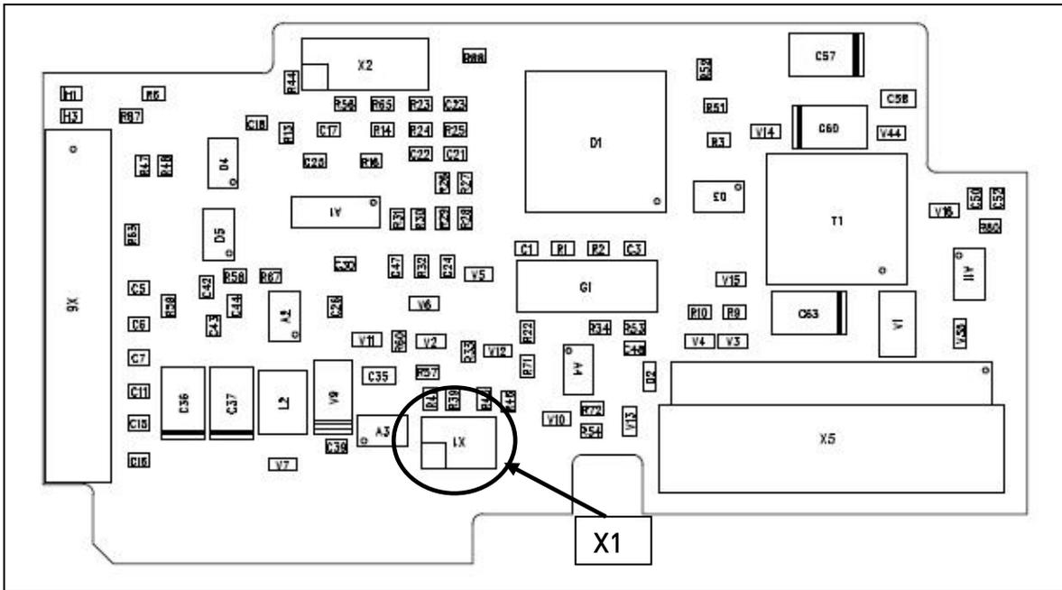
*Description:* Encoder board for **Vacon NXP** with an input for *Sin/Cos* type encoder. Programmable control voltage.
