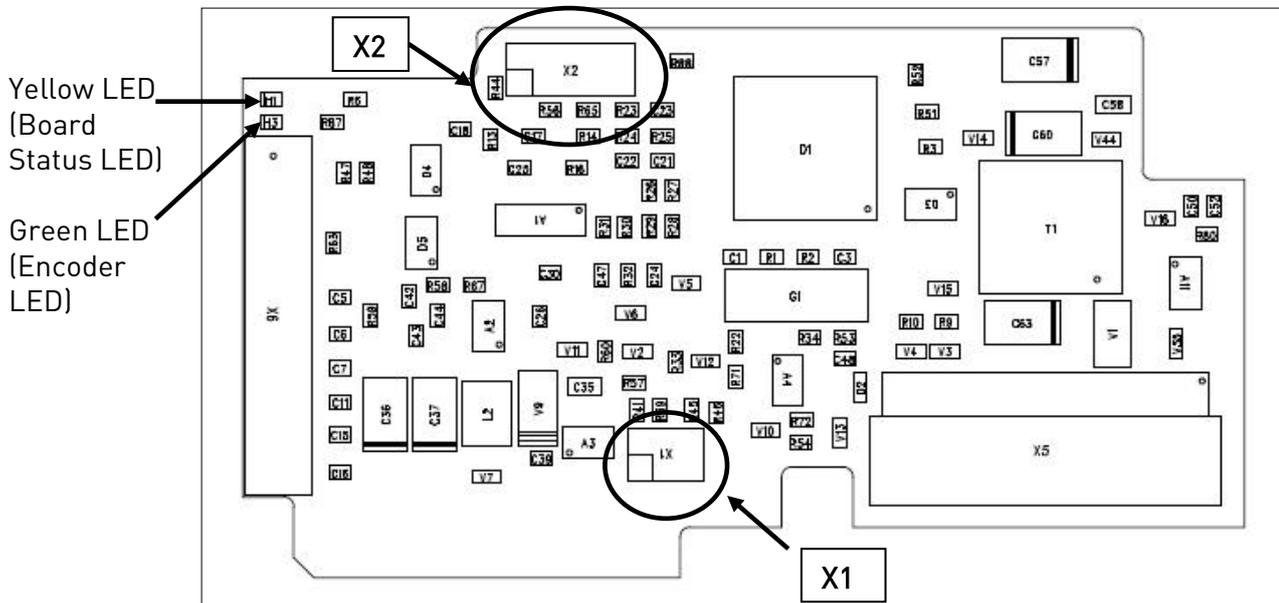
*Description:* Encoder board for **Vacon NXP** with an input for *EnDat/SSI* absolute encoder and *Sin/Cos* type encoder.
