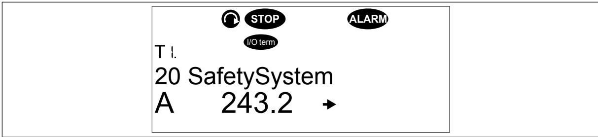
Fig. 72: Fault presentation in the fault lists. The source and fault number are shown as "source.number" (instead of "T1->T16" for other faults).
