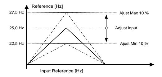
If minimum and maximum are not equal to zero adjustment is not at the middlepoint of analogue input or at zero point if -10...+10 Vdc input is used. Below picture minimum is 20 % and maximum 10 %.
