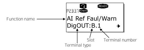
**Example**: You want to connect the digital output function *Reference fault/warning* (parameter 2.3.3.7) to the digital output DO1 on the basic board NXOPTA1 (see Vacon NX User's Manual, Chapter 6.2).
