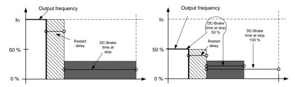
Figure 8-13. DC-braking time when Stop mode = Coasting, from nominal speed and 50 % of nominal speed.
