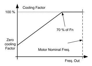
P2.12.5.5 Motor thermal protection: Time constant ID707 "MTP Motor T"
