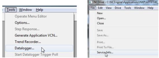
Figure 2. Datalogger window opening and Service Info upload.
