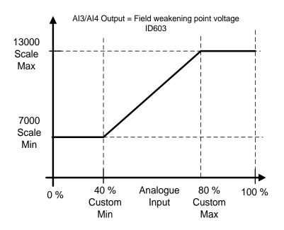
Now analogue input 3 signal 0 V to 10 V (0 mA to 20 mA) will control the field weakening point voltage between 70,00 % - 130,00 %. When setting the value remember that decimals are handled as integers.
