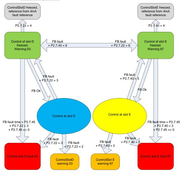
Figure: Redundant PB
