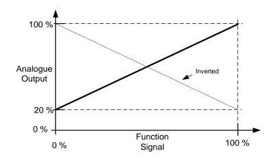
P2.5.2.6Analogue output scaleID311"lout Scale"P2.5.3.6Analogue output 2 scalingID476"lout 2 Scale"P2.5.4.6Analogue output 3 scalingID483"lout 3 Scale"
