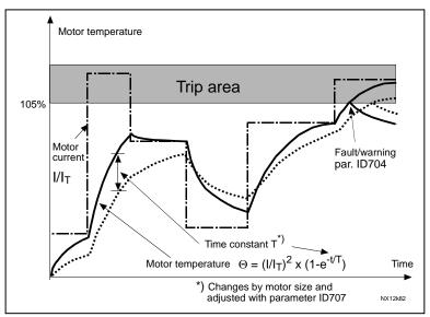
Figure 8-16. Motor temperature calculation
