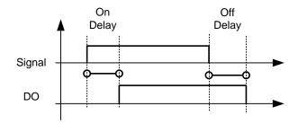
Figure 8-10. Digital outputs 1 and 2, on- and off-delays
