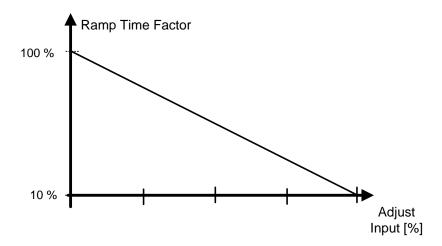
Figure 8-4. Reducing acceleration and deceleration times
