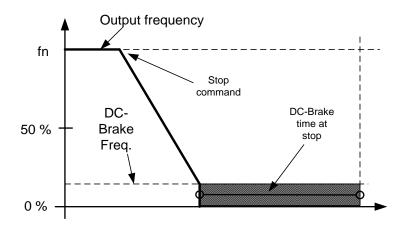
Figure 8-14. DC-braking time when Stop mode = Ramp
