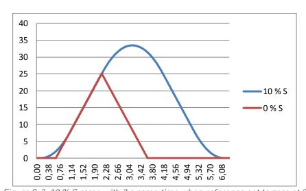
Figure 8-3. 10 % S ramp with 3 s ramp time when reference set to zero at 25 Hz
