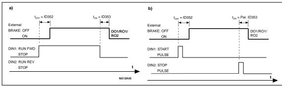
Figure 8-17. External brake control:
