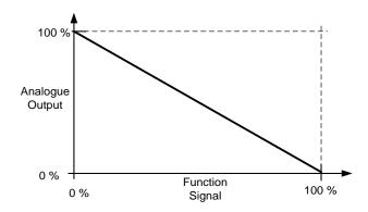
P2.5.3.5 Analogue output 2 minimum ID475 P2.5.4.5 Analogue output 3 minimum ID482
