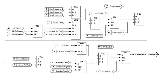
Speed reference chain before ramp control
