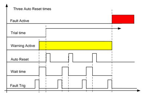
Figure 8-18. Example of Automatic restarts with three restarts
