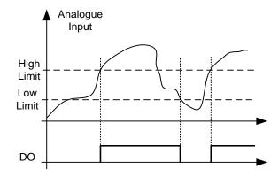
Figure 8-12. An example of On/Off-control
