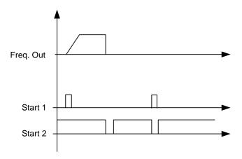
Figure 8-7. Start pulse/ Stop pulse.
