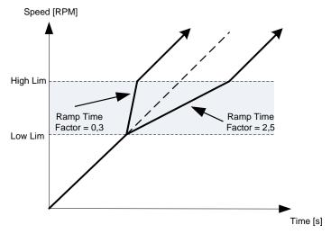
Figure 8-1. Ramp rate scaling between prohibit frequencies
