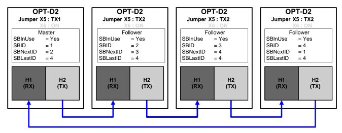
Figure 8-15. System bus physical connections with the OPT-D2 board
