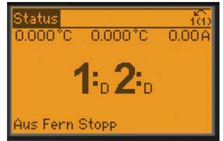
The compressor status can be read directly from the display. D = Variable speed control, O = Off, R = Mains operation, X = Deactivated
