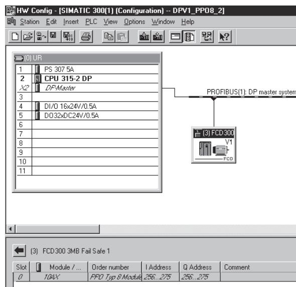
Select an I/O address in your Simatic S7 PLC. By double clicking the first module (4AX in the DP-Slave) in the Slave Station, you can either select the address in the Simatic S7 PLC or use the default addresses.
