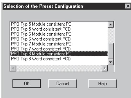
The selected PPO type can be seen in parameter *904 PPO type* after the Master have initialise the communication.
