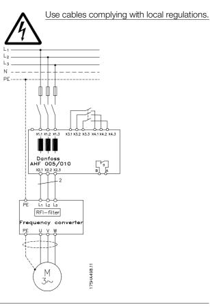
Example: Connect terminal A of the harmonic filter to terminal 12 or13 (voltage supply digital input, 24V) of the Danfoss frequency converter and terminal B to terminal 27 (digital input "Coast Inverse") the frequency converter will let go of the motor (coasting) and thereby unload the filter if a over temperature is detected.
