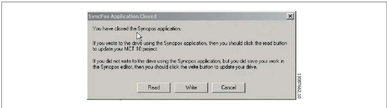
To save your changes, select Read or Write to save changes to the MCT 10 Set-up Software project or to the frequency converter, respectively. Reading or Writing can take some time.
