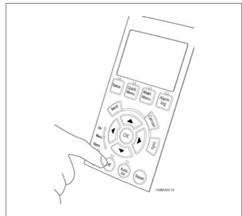
Illustration 4.22: Step 4: Power-up the unit and press the [Off] button. In this state the motor should not rotate. Press [Off] to stop the motor at any time. Note the LED at the [OFF] button should be lit. If alarms or warnings are flashing, please see chapter 7 regarding these.
