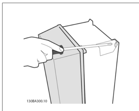
Illustration 3.14: Tightening of screws
