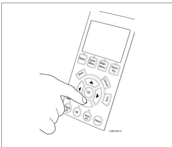
Illustration 4.45: Step 7: To move the cursor, use the left ◀ and right ▶ arrow buttons. This enables changing the speed in larger increments.
