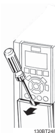
Illustration 4.46: Access to control terminals for A2, A3, B3, B4, C3 and C4 enclosures
