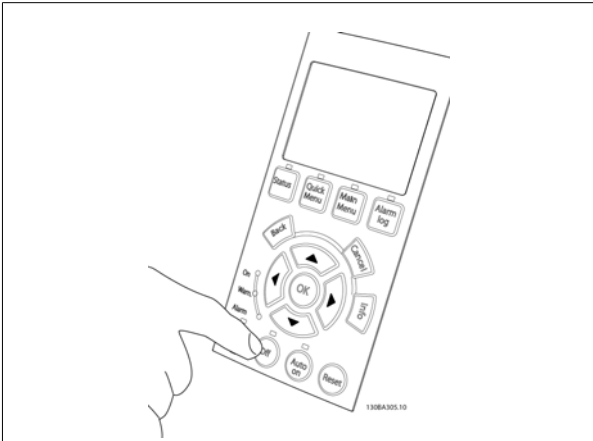
Figure 4.22: Step 4: Power up the unit and press the [Off] button. In this state, the motor should not rotate. Press [Off] to stop the motor at any time. Note that the LED on the [OFF] button should be lit. If alarms or warnings are flashing, please see chapter 7 for more information.
