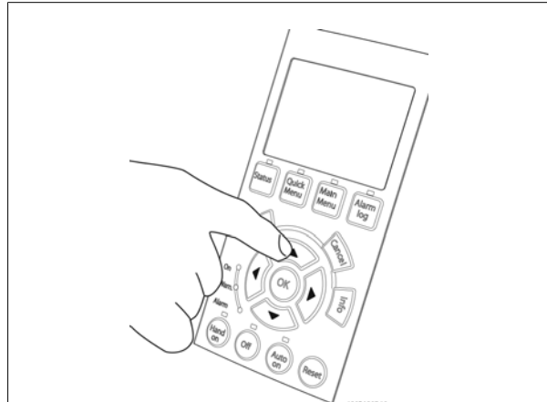
Figure 4.24: Step 6: The speed of the motor can be seen in the LCP. It can be adjusted by pushing the up ▲ and down ▼ arrow buttons.
