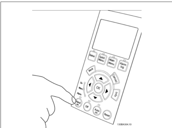
Figure 4.23: Step 5: By pressing the [Hand on] button, the LED above the button should be lit and the motor may rotate.
