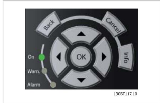
**Operation Keys** for local control are found at the bottom of the control panel.
