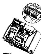
Terminals for relay connection (A5, B1 and B2 enclosures).
