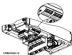
Terminals for relay connection (A2 and A3 enclosures).
