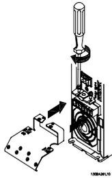
Illustration 4.3: First mount the two screws on the mounting plate, slide it into place and tighten fully.
