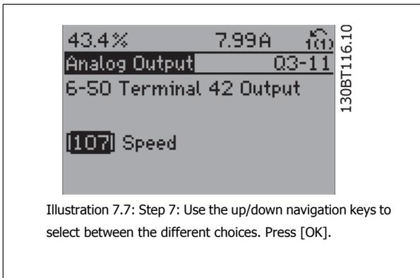
Illustration 7.7: Step 7: Use the up/down navigation keys to select between the different choices. Press [OK].
