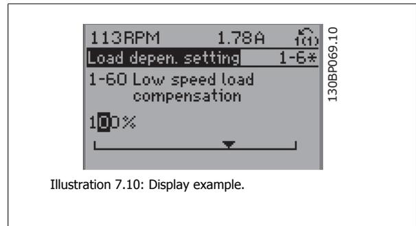
Use the up/down navigation keys to change the data value. The up key enlarges the data value, and the down key reduces the data value. Place the cursor on the value to be saved and press [OK].
