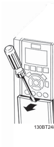
Figure 4.38: Access to control terminals for A2, A3, B3, B4, C3 and C4 enclosures
