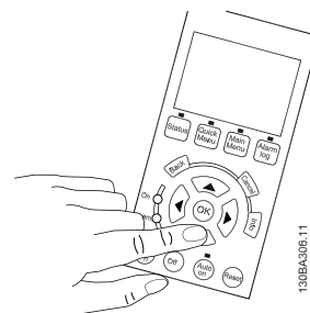
Figure 4.47: Step 7: To move the cursor, use the left ◀ and right ▶ arrow buttons. This enables speed changes by larger increments.
