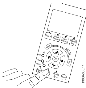
Figure 4.44: Step 4: Power up the unit and press the [Off] button. In this state, the motor should not rotate. Press [Off] to stop the motor at any time. Note that the LED on the [OFF] button should be lit. If alarms or warnings are flashing, please see chapter 7 for more information.
