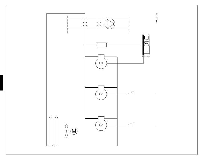
The BASIC cascade controller can also be used to control of up to three compressors for capacity control. As the compressors normally not are allowed to go below a certain speed, the compressor for variable speed control (C1) will typically be around twice the power size of the fixed speed compressors (C2 and C3).
