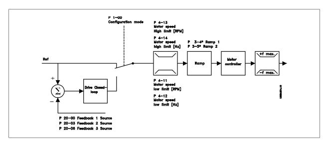
In the configuration shown in the illustration above, par. 1-00 is set to *Open-loop* [0]. The resulting reference from the reference handling system is received and fed through the ramp limitation and speed limitation before being sent to the motor control. The output of the motor control is then limited by the maximum frequency limit.
