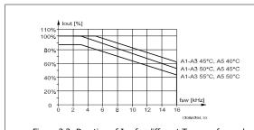
Figure 3.3: Derating of Iout for different TAMB, MAX for enclosure A, using 60 AVM and maximum 32 ft [10 m] motor cable
