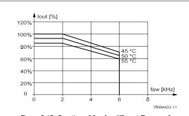
Figure 3.15: Derating of  $I_{\text{Out}}$  for different  $T_{\text{AMB, MAX}}$  for enclosure E at 480 V, using 60 AVM in normal torque mode (110% over torque)
