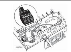
Figure 5.2: How to connect to the line supply and grounding (A5 enclosure).
