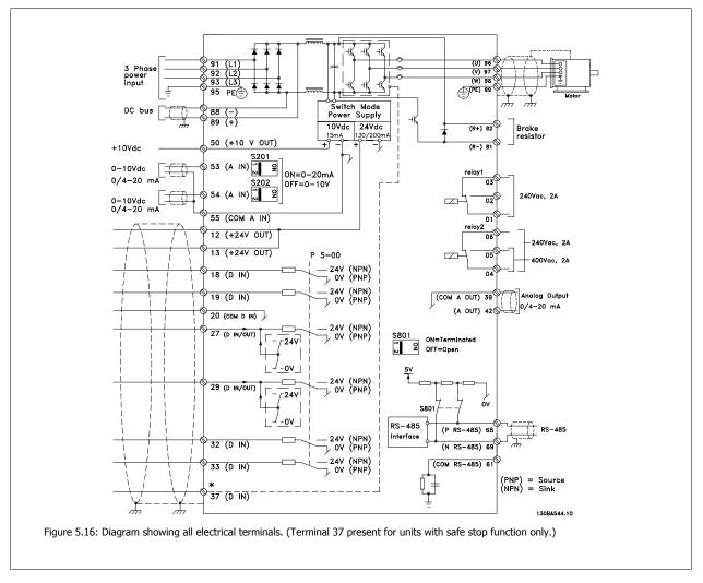
In rare cases, and depending on the installation, very long control cables and analog signals may result in 50/60 Hz ground loops due to noise from line supply cables.
