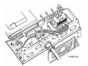
Figure 5.6: How to connect to the line supply and grounding with disconnector (A5 enclosure).
