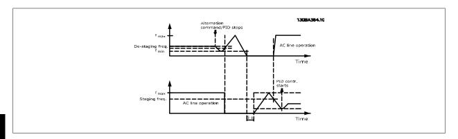
With lead pump alternation enabled, a maximum of two pumps are controlled. At an alternation command, the lead pump will ramp to minimum frequency (fmin), and after a delay, it will ramp to maximum frequency (fmax). When the speed of the lead pump reaches the de-staging frequency, the fixed speed pump will be cut out (de-staged). The lead pump continues to ramp up, then ramps down to a stop, and the two relays are cut out.
