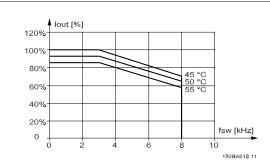
Figure 3.9: Derating of  $I_{\text{out}}$  for different  $T_{\text{AMB, MAX}}$  for enclosure D at 480 V, using 60 AVM in normal torque mode (110% over torque)
