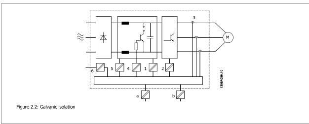
The functional galvanic isolation (a and b in drawing) is for the 24 V backup option and for the RS-485 standard bus interface.
