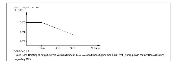
An alternative is to lower the ambient temperature at high altitudes and thereby ensure 100% output current at high altitudes.
