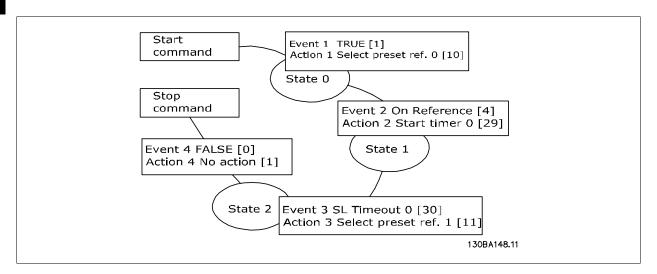
Set the smart logic control in par. 13-00 to ON.
