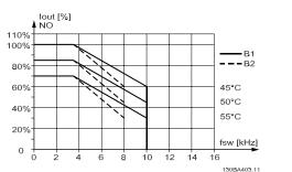
Figure 3.6: Derating of  $I_{\text{Out}}$  for different  $T_{\text{AMB, MAX}}$  for enclosure B, using SFAVM in normal torque mode (110% over torque)
