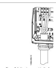
Figure 5.4: How to connect to the line supply and grounding (C1 and C2 enclosure).
