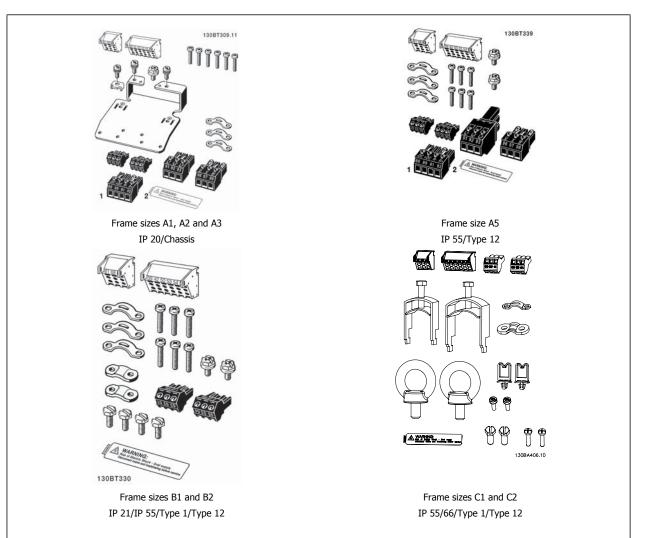
1 + 2 only available in units with brake chopper. Only one relay connector is included for FC 101/301 units. For DC link connection (Load sharing), the connector 1 can be ordered separately (Code no 130B1064).
