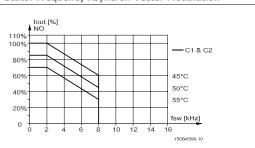
Figure 3.8: Derating of  $I_{\text{out}}$  for different  $T_{\text{AMB, MAX}}$  for enclosure C, using SFAVM in normal torque mode (110% over torque)
