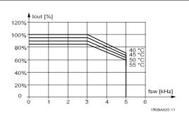
Figure 3.10: Derating of  $I_{\text{out}}$  for different  $T_{\text{AMB, MAX}}$  for enclosure D at 480 V, using SFAVM in normal torque mode (110% over torque)
