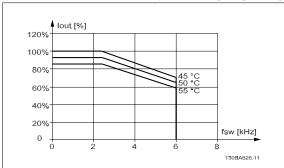
Figure 3.11: Derating of  $I_{\text{Out}}$  for different  $T_{\text{AMB, MAX}}$  for enclosure D at 600 V, using 60 AVM in normal torque mode (110% over torque). Note: *not* valid for P315.
