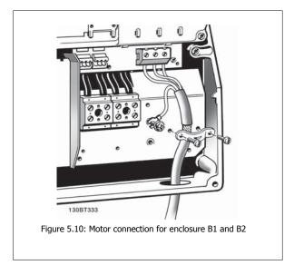
All types of three-phase asynchronous standard motors can be connected to the adjustable frequency drive. Normally, small motors are star-connected (230/400 V, D/Y). Large motors are delta-connected (400/600 V, D/Y). Refer to the motor nameplate for correct connection mode and voltage.
