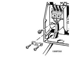
Figure 5.3: How to connect to the line supply and grounding (B1 and B2 enclosure).
