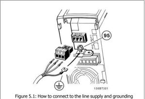
Figure 5.1: How to connect to the line supply and grounding (A2 and A3 enclosure).
