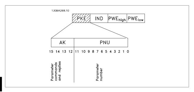
Bits no. 12-15 transfer parameter commands from master to slave and return processed slave responses to the master.
