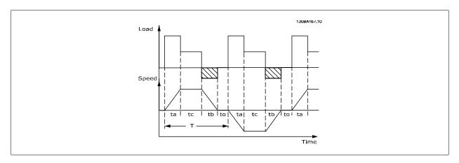
Danfoss offers brake resistors with duty cycle of 5%, 10% and 40% suitable for use with the VLT® FC102 HVAC drive series. If a 10% duty cycle resistor is applied, it is capable of absorbing braking energy up to 10% of the cycle time, with the remaining 90% being used to dissipate heat from the resistor.
