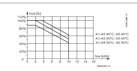
Figure 3.4: Derating of Iout for different TAMB, MAX for enclosure A, using SFAVM and a maximum of 32 ft. [10 m] motor cable
