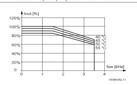
Figure 3.14: Derating of  $I_{\text{out}}$  for different  $T_{\text{AMB, MAX}}$  for enclosure D at 600 V, using SFAVM in normal torque mode (110% over torque). Note: P315 *only*.
