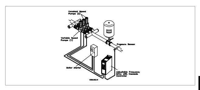
The BASIC Cascade Controller is used for pump applications where a certain pressure ("head") or level needs to be maintained over a wide dynamic range. Running a large pump at variable speed over a wide range is not an ideal solution because of low pump efficiency, and because there is a practical limit of about 25% rated full load speed for running a pump.
