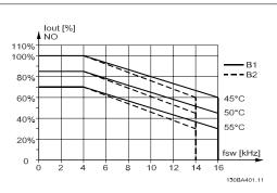
Figure 3.5: Derating of  $I_{\text{out}}$  for different  $T_{\text{AMB, MAX}}$  for enclosure B, using 60 AVM in normal torque mode (110% over torque)
