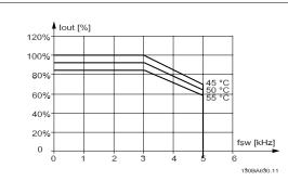
Figure 3.13: Derating of  $I_{out}$  for different  $T_{AMB, MAX}$  for enclosure D at 600 V, using 60 AVM in normal torque mode (110% over torque). Note: P315 *only*.
