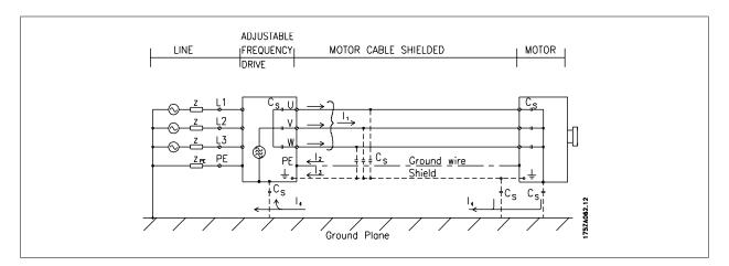
If the shield is to be placed on a mounting plate for the adjustable frequency drive, the mounting plate must be made of metal, because the shield currents have to be conveyed back to the unit. Moreover, ensure good electrical contact from the mounting plate through the mounting screws to the adjustable frequency driver chassis.
