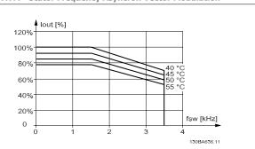
Figure 3.18: Derating of  $I_{\text{Out}}$  for different  $T_{\text{AMB, MAX}}$  for enclosure E at 600 V, using SFAVM in normal torque mode (110% over torque).
