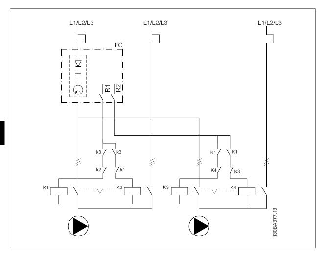
Every pump must be connected to two contactors (K1/K2 and K3/K4) with a mechanical interlock. Thermal relays or other motor protection devices must be applied according to local regulation and/or individual demands.
