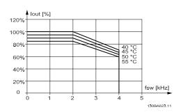
Figure 3.16: Derating of  $I_{\text{Out}}$  for different  $T_{\text{AMB, MAX}}$  for enclosure E at 480 V, using SFAVM in normal torque mode (110% over torque)
