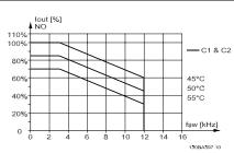
Figure 3.7: Derating of  $I_{\text{out}}$  for different  $T_{\text{AMB, MAX}}$  for enclosure C, using 60 AVM in normal torque mode (110% over torque)
