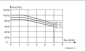
Figure 3.17: Derating of  $I_{\text{out}}$  for different  $T_{\text{AMB, MAX}}$  for enclosure E at 600 V, using 60 AVM in normal torque mode (110% over torque).
