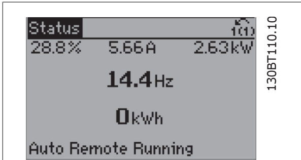
Figure 2.7: Step 1: Turn on the adjustable frequency drive (yellow LED lights)
