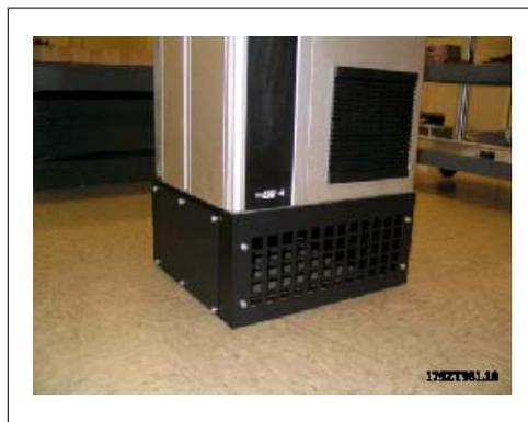
Illustration 3.67: Frame D2 with pedestal installed
