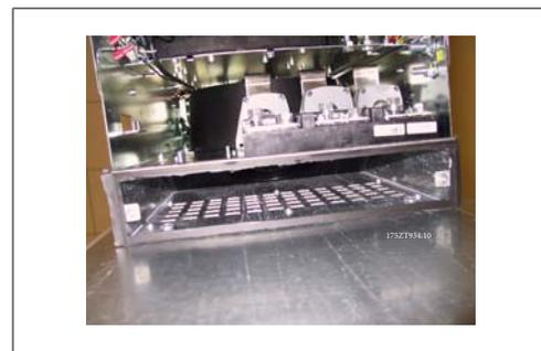
Illustration 3.33: Bottom duct adapter installed
