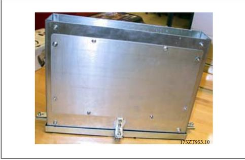
The duct assembly is used to mark the bottom cutout. Temporarily install the bottom duct work as shown to the right. Use the inside of the ductwork to mark the bottom of the enclosure for the opening.
