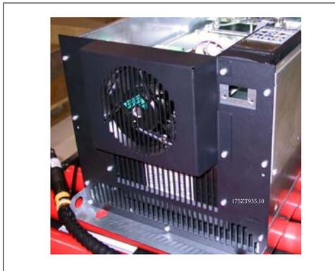
Illustration 3.35: Top of IP 00 / Chassis frequency converter
