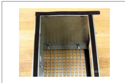
3.43: The gasket applied to both sides of the adjustable frequency drive bracket and duct vented-top cover.
