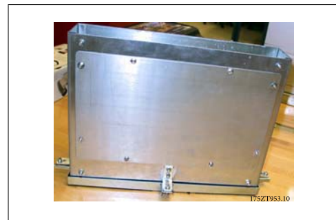
3.53: Completely assembled bottom duct work
