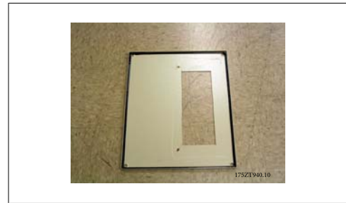
3.40: Rittal enclosure top with cut-out The standard Rittal enclosure top is cut. The gasket is not used on the cut-out. The gasket is part of the duct work.
