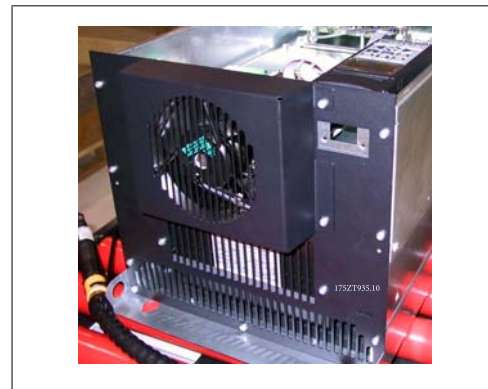
3.35: Top of IP 00/Chassis adjustable frequency drive
