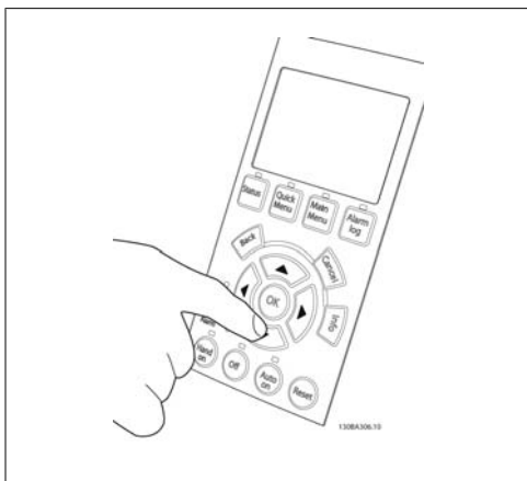
Illustration 5.25: Step 7: To move the cursor, use the left ◀ and right ▶ arrow buttons. This enables changing the speed in larger increments.
