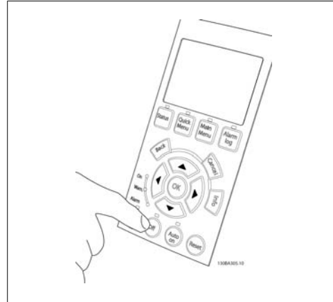
Illustration 5.26: Step 8: Press the [Off] button to stop the motor again.
