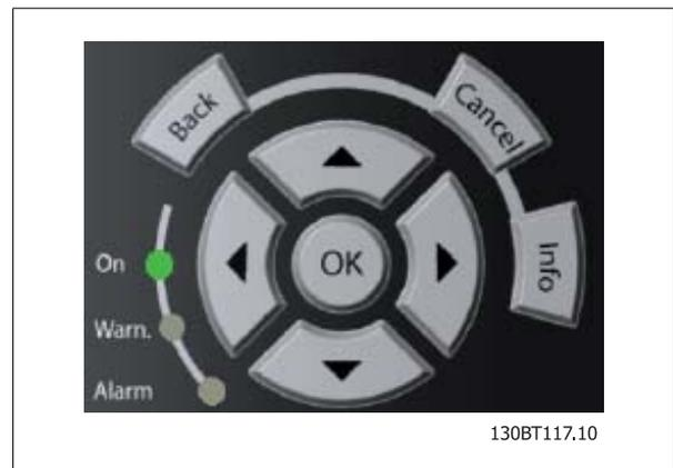
**Operation Keys** for local control are found at the bottom of the control panel.
