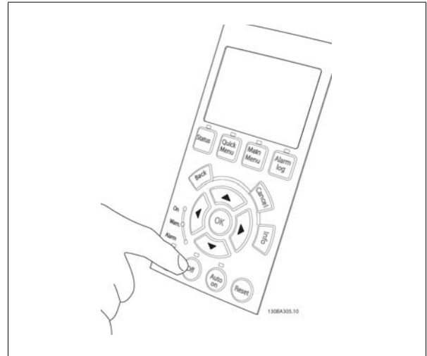
Illustration 5.53: Step 8: Press the [Off] button to stop the motor again.
