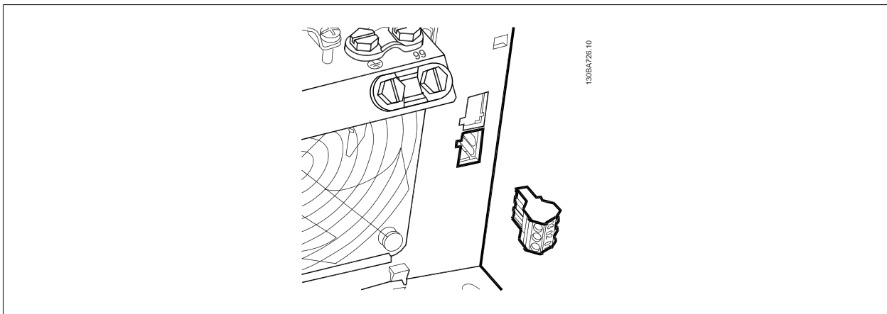
Illustration 5.22: Terminals for relay connections for B3. Only one knock-out is fitted from the factory.
