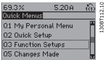
Figure 1.9: Step 3: Use the up/down navigation keys to scroll down to Function Set-ups. Press [OK].
