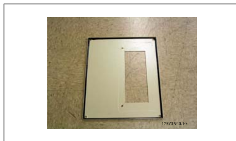
Illustration 3.40: Rittal enclosure top with cutout Standard Rittal enclosures top is cut. Gasket is not used on the cutout. Gasket is part of duct work.
