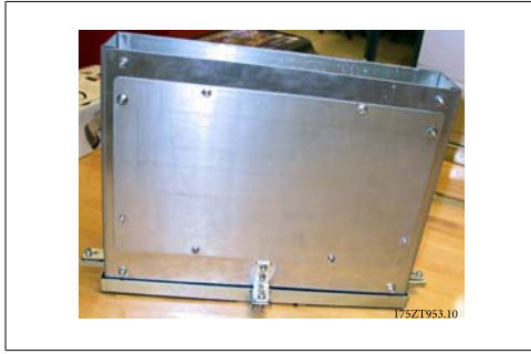
Illustration 3.53: Completely assembled bottom duct work
