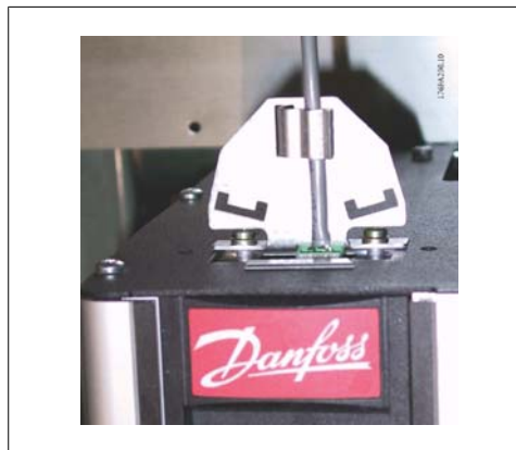
Illustration 3.69: Top connection for fieldbus.
