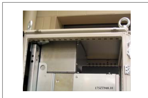
3.49: Enclosure top installed
