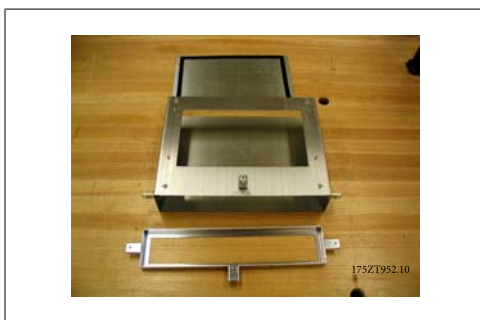
3.52: Bottom duct work partially assembled
