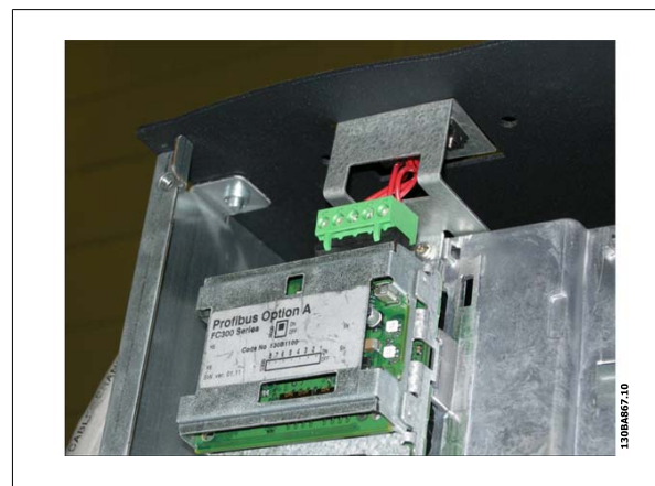
Illustration 3.55: Top connection for fieldbus.
