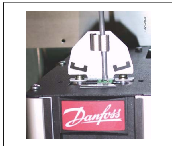
Illustration 6.36: Top connection for fieldbus.
