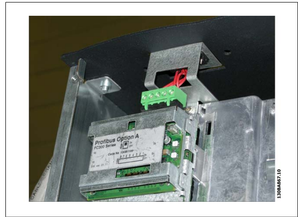
Illustration 8.36: Top connection for fieldbus.
