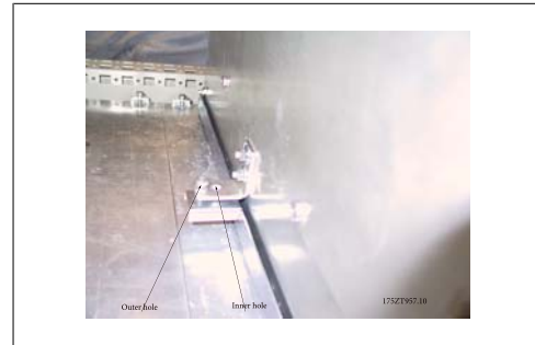
Illustration 3.58: Move mounting screws from the outer hole to the inner hole
