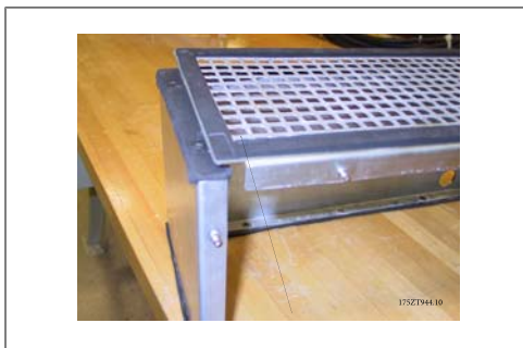
Illustration 3.41: Gasket folds over the edge to form seal between the duct and top vented cover
