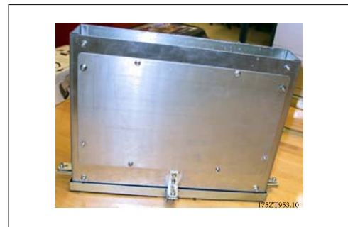
3.53: Completely assembled bottom duct work
