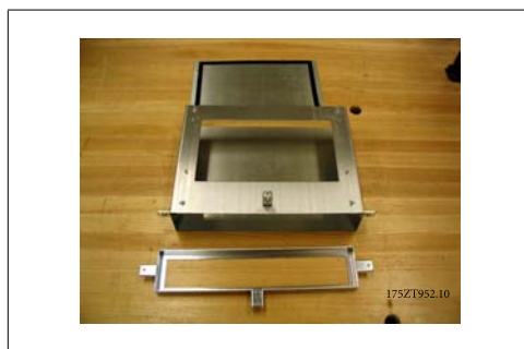
3.52: Bottom duct work partially assembled
