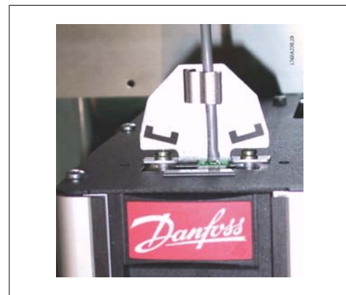
3.69: Top connection for the serial communication bus.
