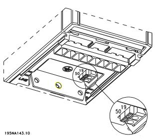
The thermistor must be connected between terminal 50 (+10V) and one of the digital inputs 18, 19, 27 and 29.
