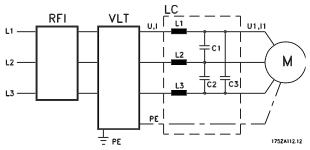
When a motor is controlled by a frequency converter, at times you will be able to hear the acoustic noise from the motor. The noise, which is caused by the design of the motor, is generated every time one of the inverter contacts in the frequency converter is activated. The frequency of the acoustic noise therefore corresponds to the frequency converter's connection frequency.
