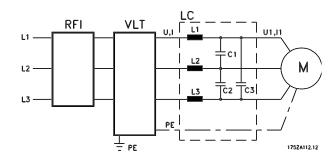
Because of the ripple current in the coils there will be some noise from the coils. However, if the filter is built into a cabinet or the like the coil noise will be no problem.
