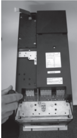
6.Loosen the terminal bracket with a screwdriver.
