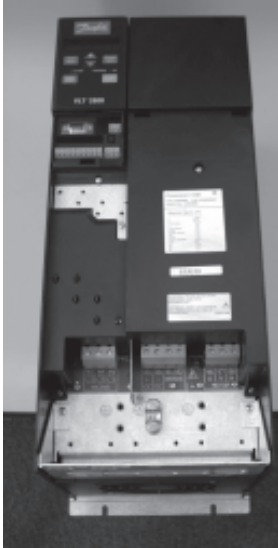
1. VLT 2880-2882 after removal of front cover.
