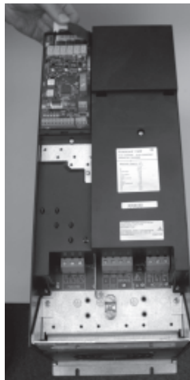
3.Remove flat cable of the control card.
