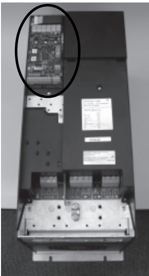
2.Remove control card cover.
