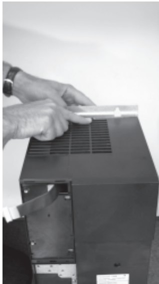
9.Push on the top of the VLT to remove cover.
