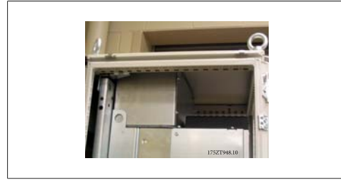
Illustration 4.21: Enclosure top installed
