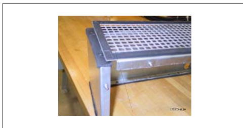
Illustration 4.13: Gasket folds over the edge to form seal between the duct and top vented cover
