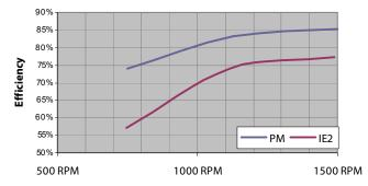
Shown efficiency curves are measured on a 1,1 kW PM and IE2 motor at VT (variable torque) load.
