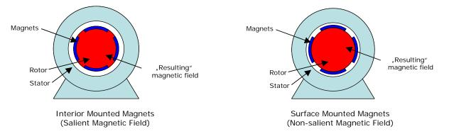
The most common are surface mounted magnets. If the nameplate does not provide values for Lg and Ld, contact the motor supplier for a data sheet to determine the motor type. Currently Danfoss supports non-salient motor types only.
