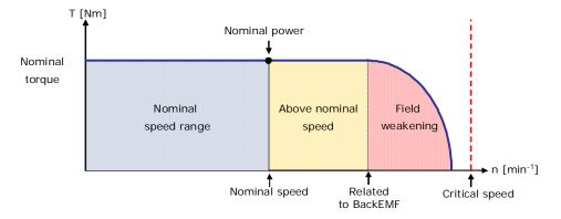
The required voltage at the nominal load point is typically below the supplied mains voltage (e.g. 320V on 400V mains) for many PM motors. Therefore many PM motors can be operated above the nominal power rating.
