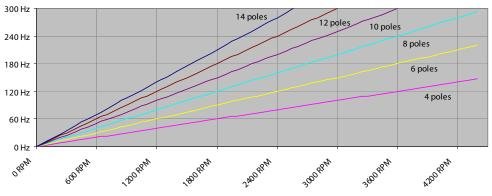
Relation between actual motor frequency, number of poles and resulting speed (60 Hz oriented)
