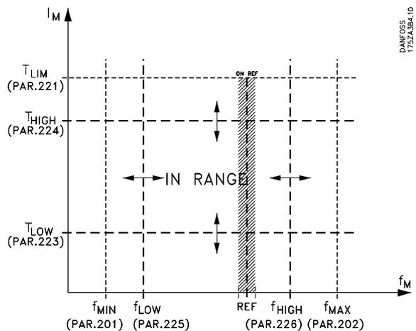
**222 Torque limit for generating operation (TORQ LIMIT GENER)**
