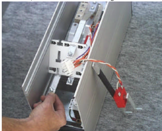
Step 6. Slide the busbar (up or down depending on the model) until clear of the SCR fixing screws.
