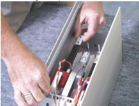
Step 5. Undo the screw (1) connecting the output bus bar (T1, T2 or T3) to the top of the SCR being replaced.
