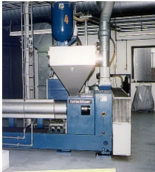
Fig. 1 shows a typical screw extruder for plastics processing. The raw materials enter the extruder in the feed section and the rotating screw moves the material forward to the compression section. In this zone the pressure builds up and the friction between the granulated particles plasticates the material. In the metering section the liquid material is pushed to the die.
