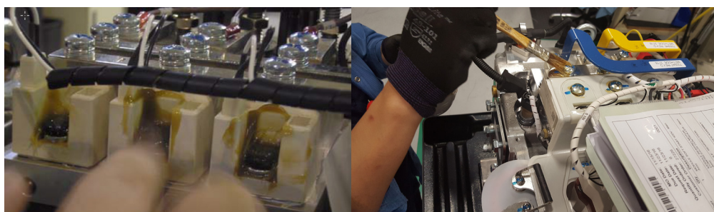
Figure 107 - SCR Screw Dielectric Grease Application
