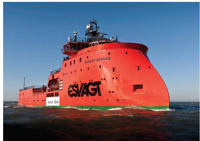
The standby safety vessel "Esvagt Bergen" is equipped with a SEM-SAFE® high-pressure water mist fire fighting system.
