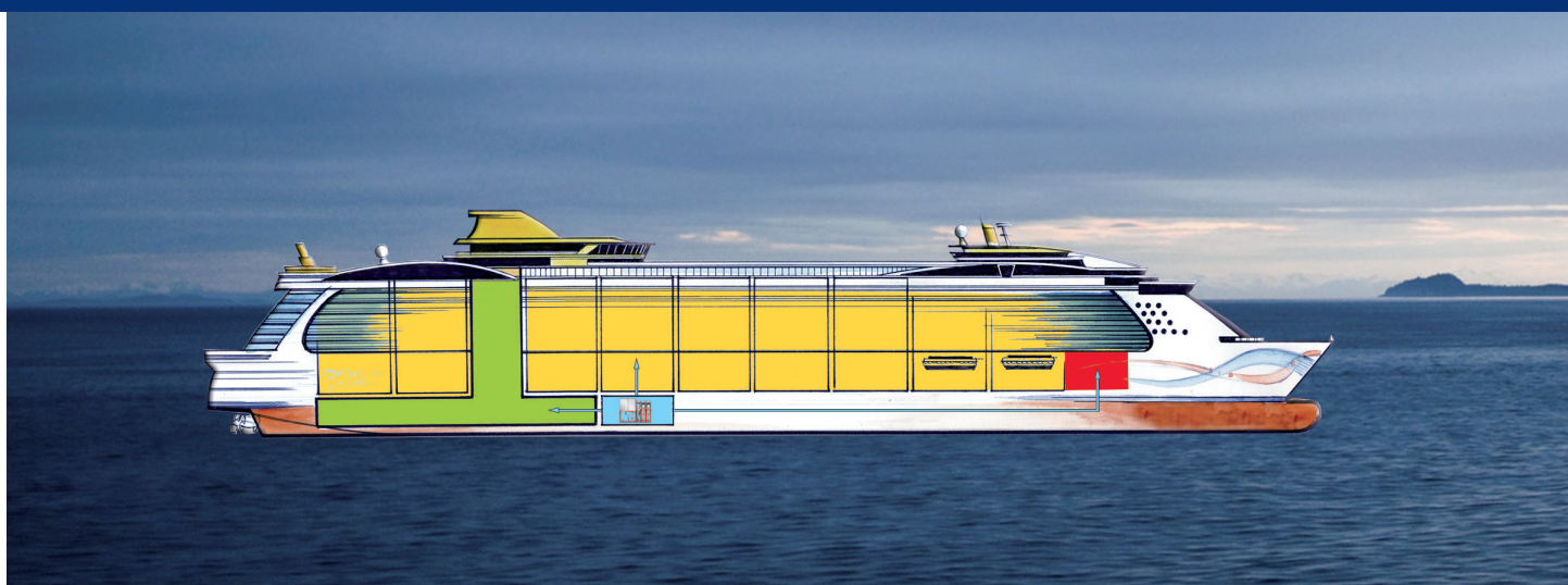
■ Sem-Safe® Pump Unit ■ Engine room, Total Flooding and Local Application ■ Accommodation ■ Deep Fat fryer and Duct in Galley
